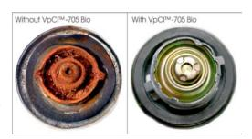
VpCI<sup>™</sup>-705 Bio from Cortec<sup>®</sup> Corporation is a unique fuel stabilizer that provides vapor corrosion protection at a very low dosage. A comparison test on tank gaskets (above) shows the protection benefits of using VpCI<sup>™</sup>-705 Bio.
